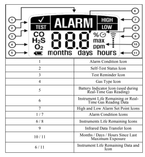
When gas is present, the display screen will automatically shift to a display that shows gas concentration and a battery icon.
